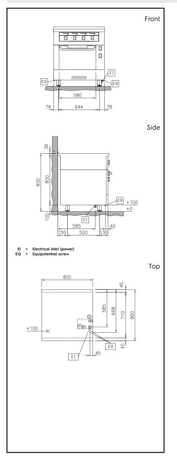
Modular Cooking Range Line thermaline 80 - 4 Zone Induction Top on Oven, 1 Side with Backsplash H=800 The company reserves the right to make modifications to the products without prior notice. All information correct at time of printing.
